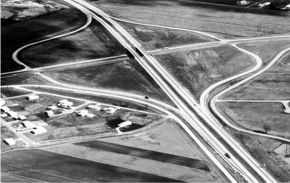
Exhibit 10-20. Existing Four-Leg Interchange With Diamond Stage Construction
