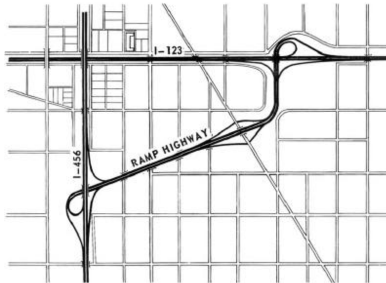
Exhibit 10-38. Offset Interchange via Ramp Highway
