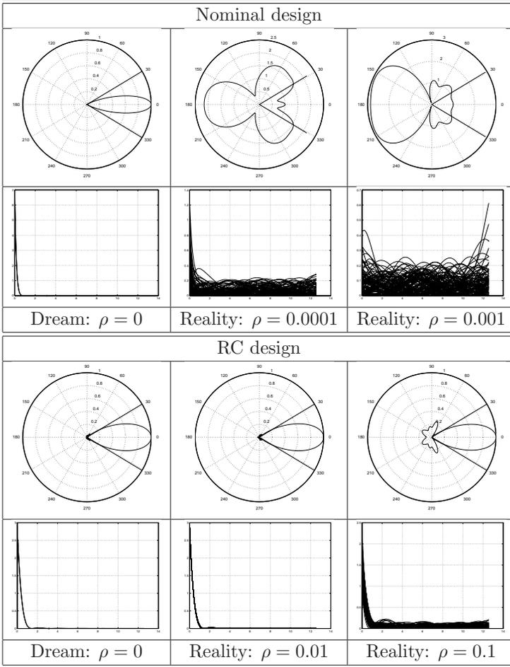
Figure 7.1 Nominal and RC antenna designs. First rows: sample plots of  $|D(\phi)|$  in polar coordinates; the diagrams are normalized to have  $D(0) = 1$ . Second rows: bunches of 100 simulated energy densities, cf. section 3.3.
