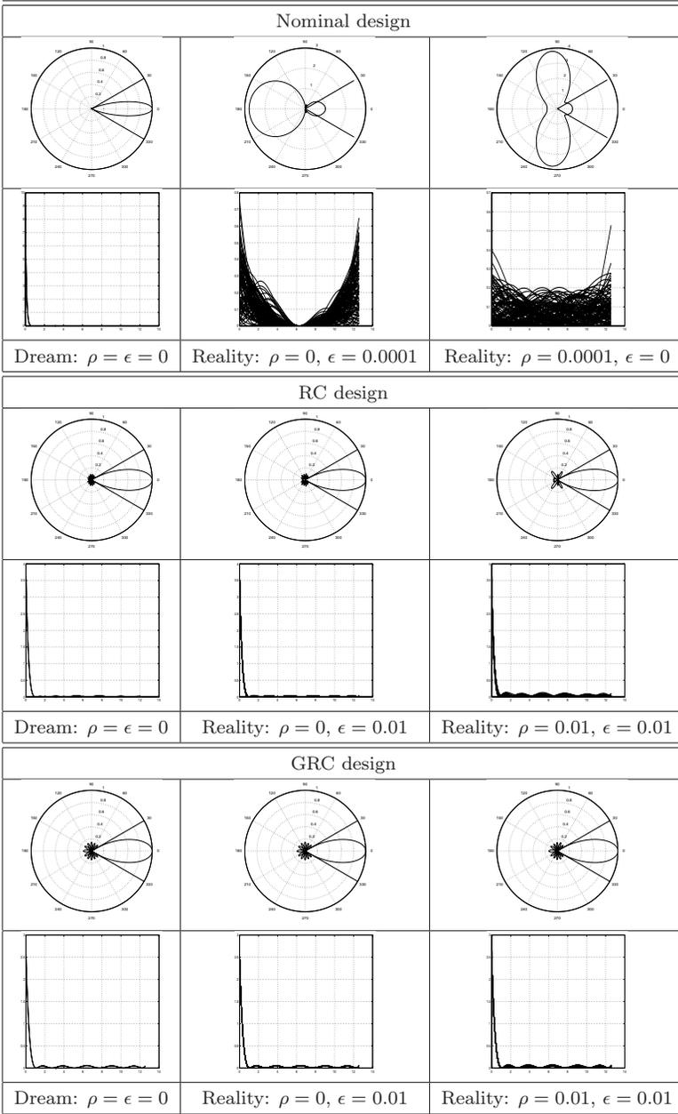
Figure 3.1 Nominal, RC and GRC antenna designs. First rows: sample plots of  $|D(\phi)|$  in polar coordinates; the diagrams are normalized to have  $D(0) = 1$ . Second rows: bunches of 100 simulated energy densities.
